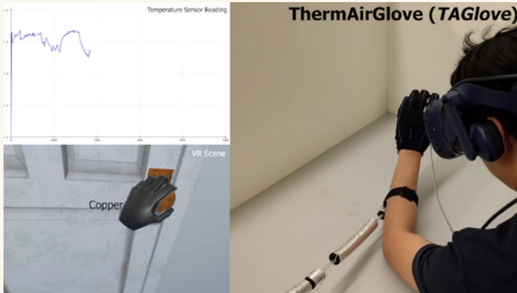
The user touches the door handle made of copper in VR, with ThermAirGlove on his hand. He can then feel the cooling feedback of touching metal just like in the real world
