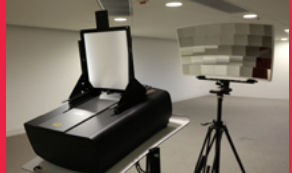
An autostereoscopic 3D display based on mirror array developed by Dr. Lam's research group
