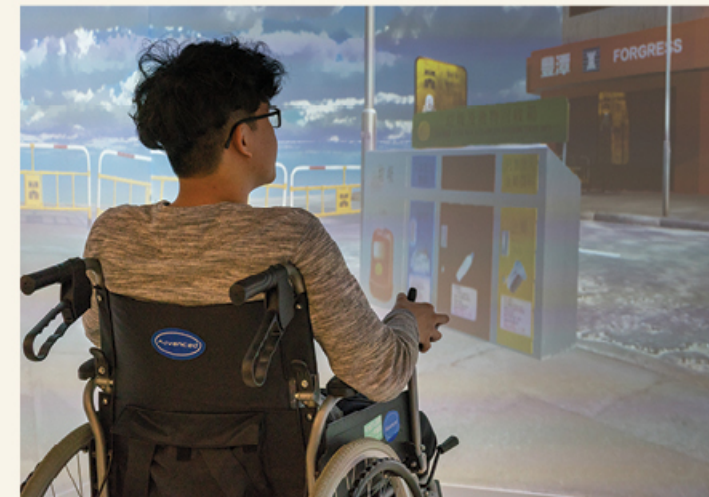
Cave Automatic Virtual Environment (CAVE) display test. CAVE is an immersive technology that uses three or more projections or displays to build a virtual environment surrounding the user to enhance the immersion while interacting with the 3D environment
